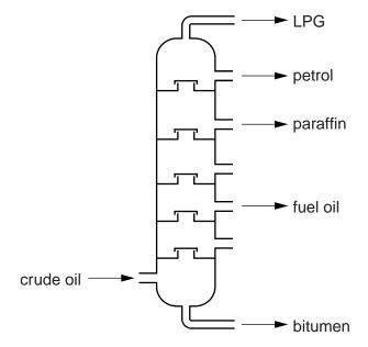
(a) What is the name of the process that separates crude oil into fractions?
